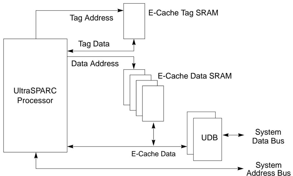
Figure 1-2 UltraSPARC Subsystem
