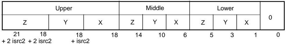
Figure 13-17 Three Dimensional Array Blocked-Address Format (Array16)
