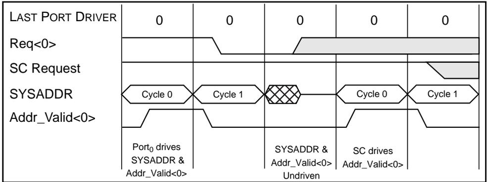
Figure 7-15 Arbitration: SC Arbitrates and Sends a Packet to Port<sub>0</sub>
