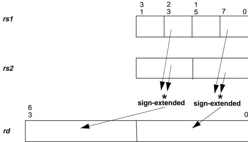
Figure 13-14 FMULD8ULx16 Operation
