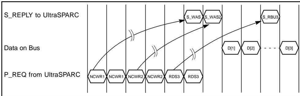
Figure 7-28 S\_REPLY Pipelining to UltraSPARC for Data Transfers
