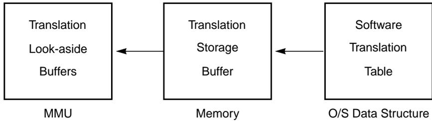
Figure 4-3 Software View of the UltraSPARC MMU
