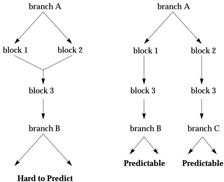
Figure 16-10 Branch Transformation to Reduce Mispredicted Branches
