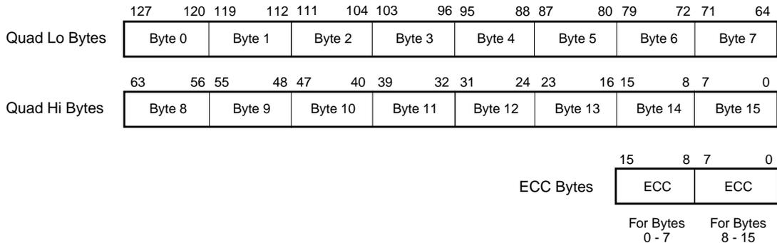
Figure 7-2 Data and ECC Byte Addresses Within a Quadword
