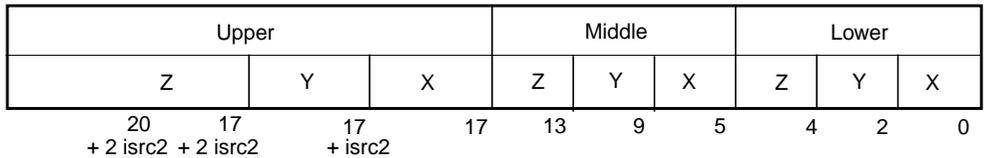
Figure 13-16 Three Dimensional Array Blocked-Address Format (Array8)
