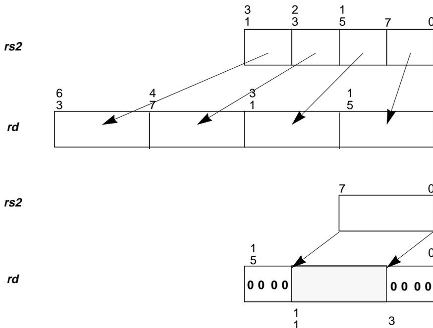
Figure 13-6 FEXPAND Operation
