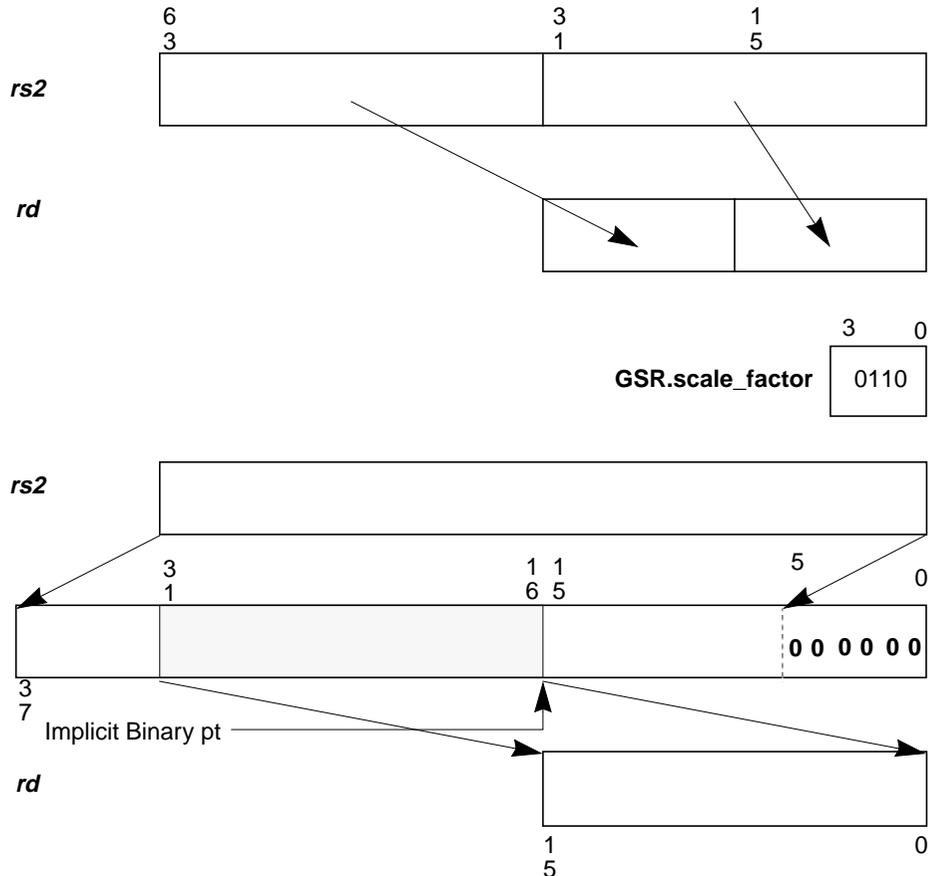
Figure 13-5 FPACKFIX Operation
