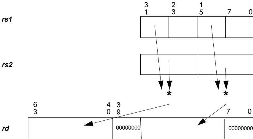
Figure 13-13 FMULD8SUx16 Operation
