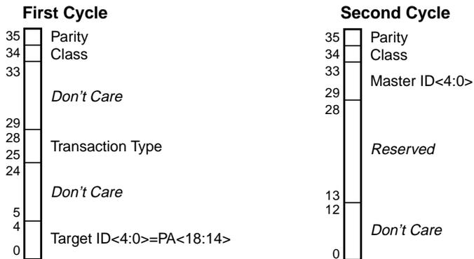
Figure 7-34 Packet Format: P\_INT\_REQ Transaction
