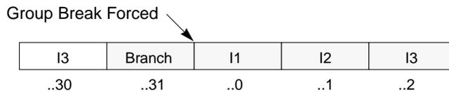
Figure 16-5 Artificial Branch Inserted after a 32-byte Boundary
