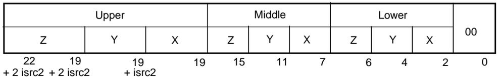
Figure 13-18 Three Dimensional Array Blocked-Address Format (Array32)
