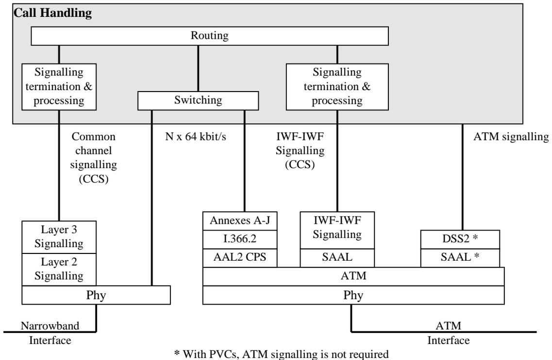
**Figure 7: Protocol Reference Model for switched trunking with CCS interface and CCS over AAL5 between IWFs**
