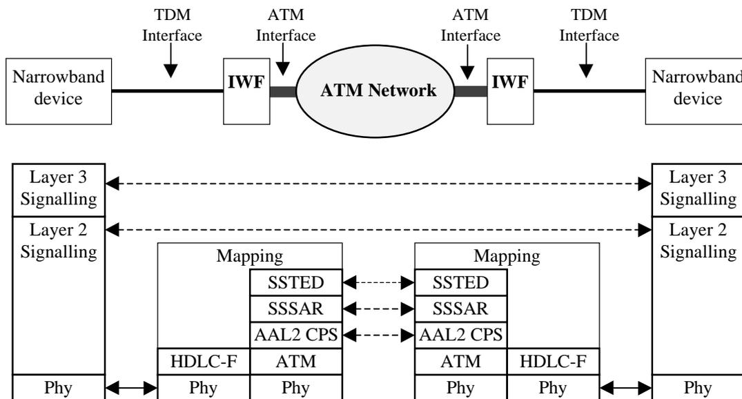
**Figure 15: Transparent transport of CCS information using AAL2**
