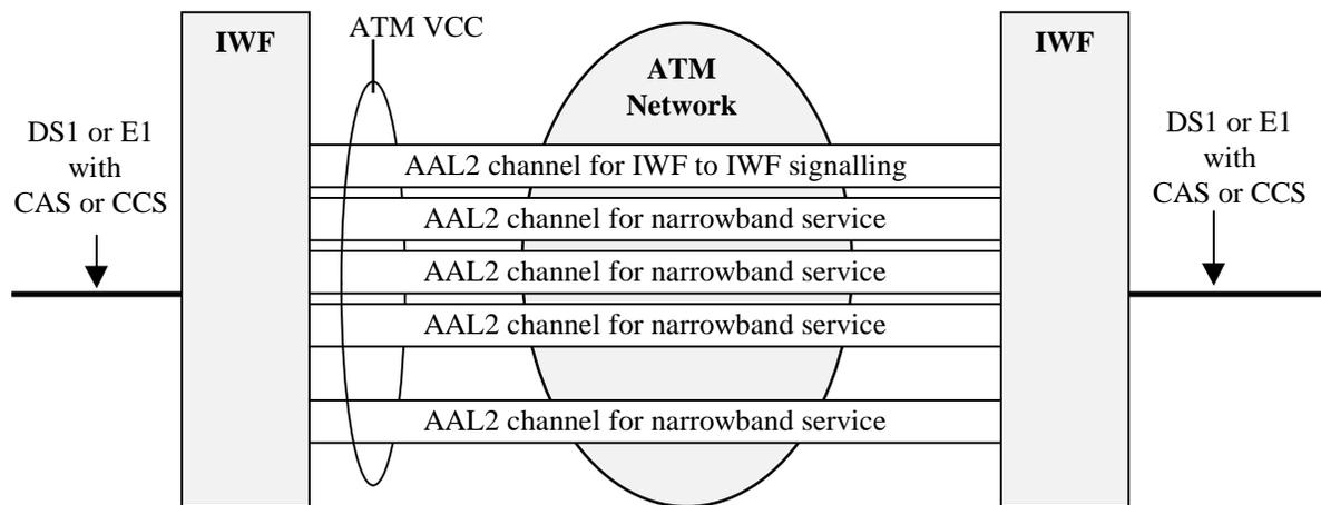
**Figure 13: AAL2 Channels within an ATM VCC**
