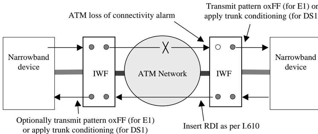
**Figure 18: ATM VCC fault detection**
