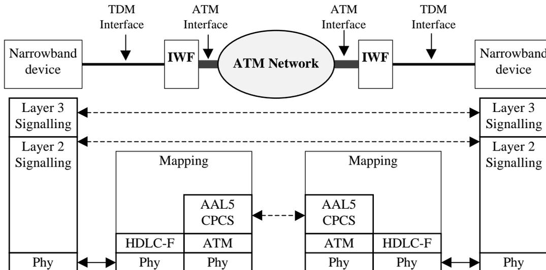
**Figure 14: Transparent transport of CCS information using AAL5**
