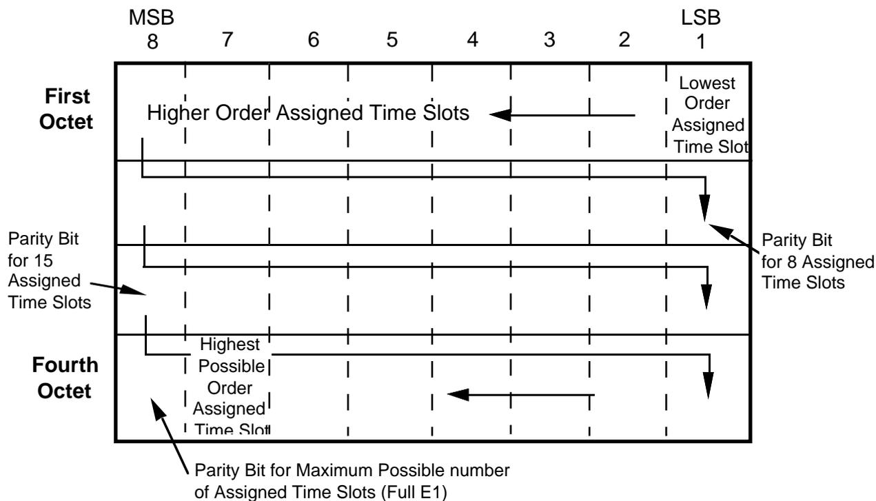
**Figure 3.4 Bitmask Format**
