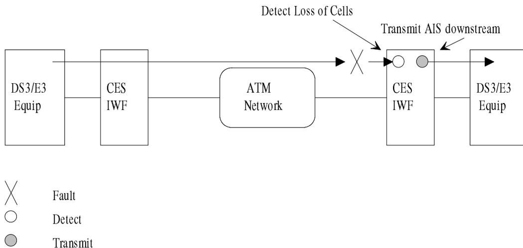
**Figure 4-3: Unstructured DS3/E3 Virtual Channel Fault Indication**
