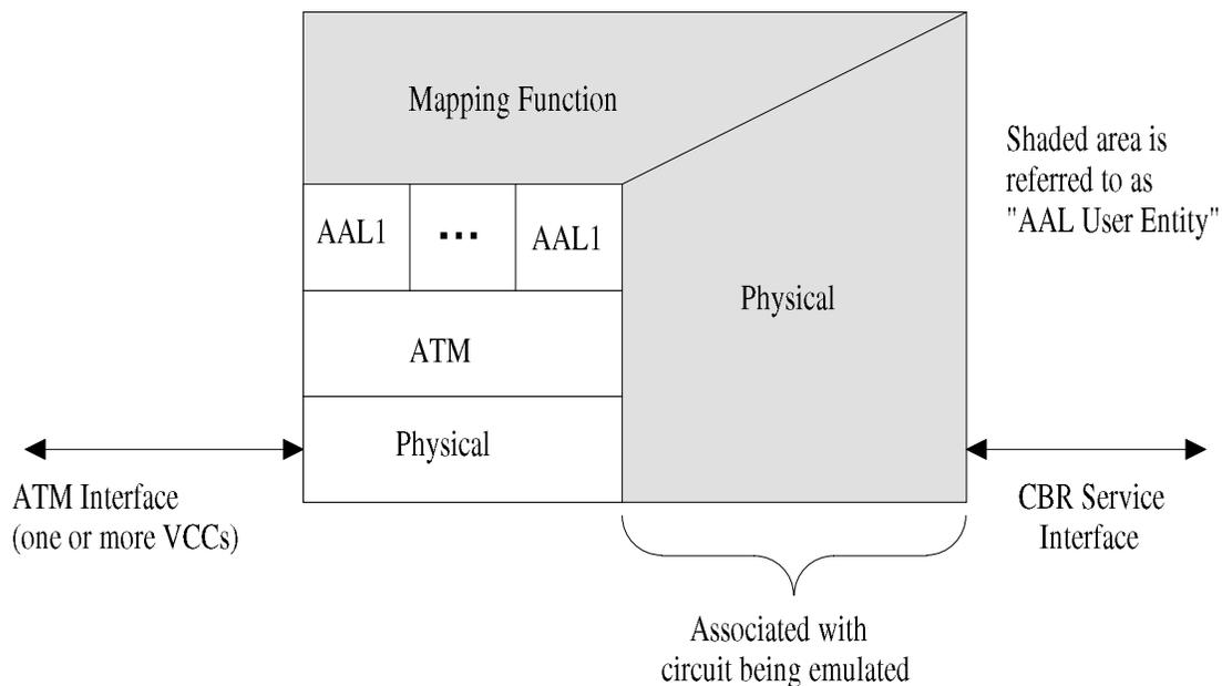
**Figure 2-2: DS1/E1/J2 Structured Service Interworking Function - Layering Perspective**
