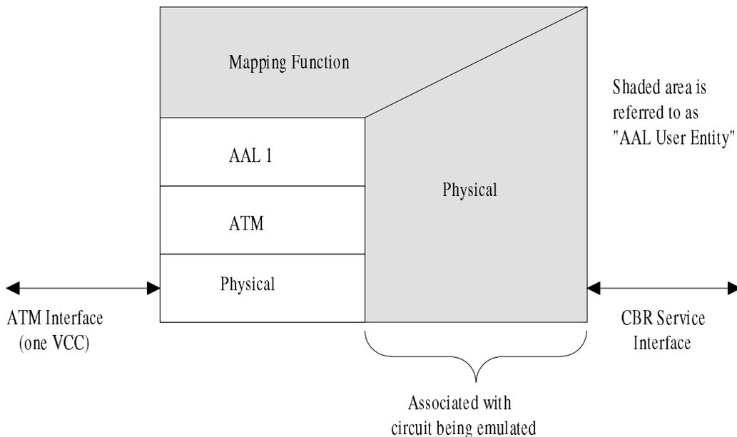
**Figure 4-1: Unstructured DS3/E3 Service Interworking Function -- Layering Perspective**
