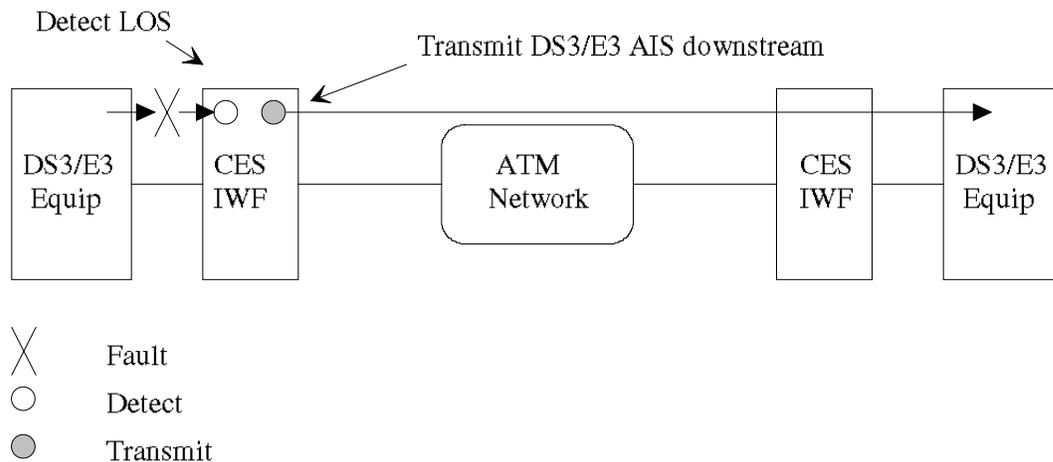
**Figure 4-2: Unstructured DS3/E3 Service Interface Fault Indication**
