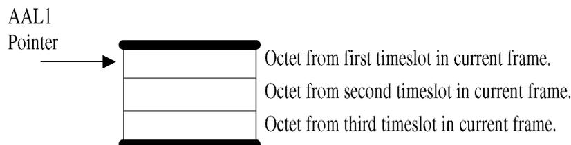
**Figure 2-5: Example Singleframe Structure Format for 3x64 kbit/s**
