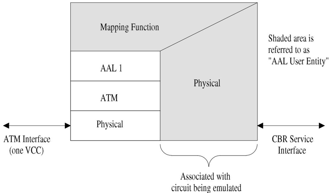
**Figure 3-1: DS1/E1/J2 Unstructured Service Interworking Function - Layering Perspective**
