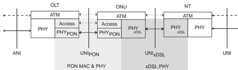
**Figure 3-6 PON Transport Protocol Mapping**
