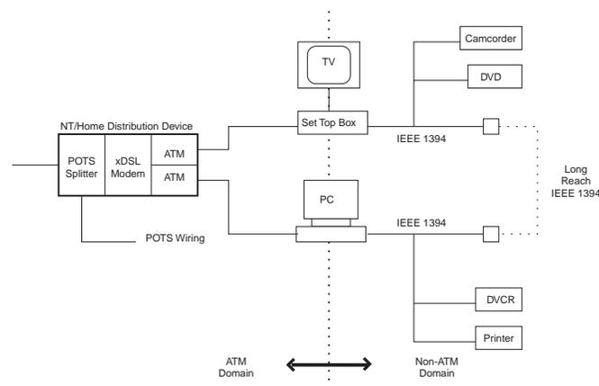
**Figure A-4 Connection between ATM and non ATM home networks**
