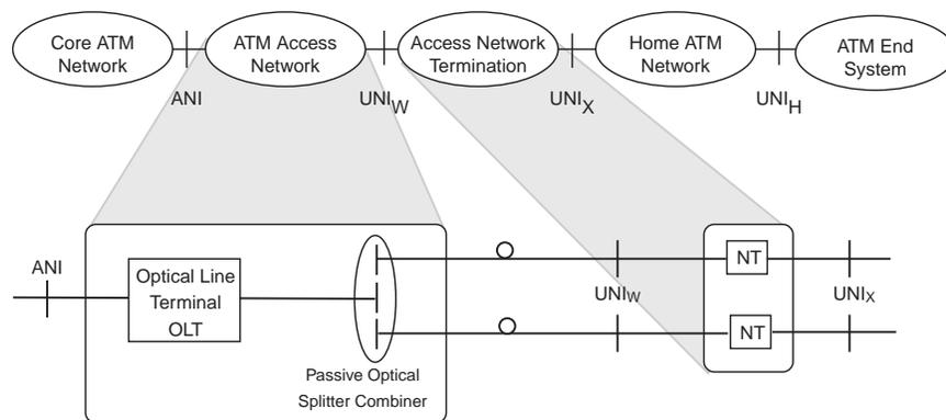
**Figure 3-3 ATM over FTTH using PON Reference Architecture**
