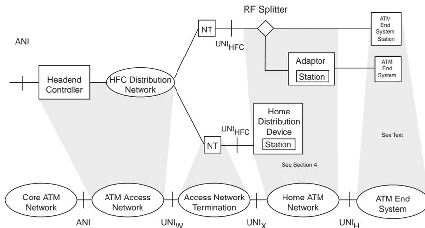
**Figure 3-1 ATM Over HFC Passive NT Reference Architecture**
