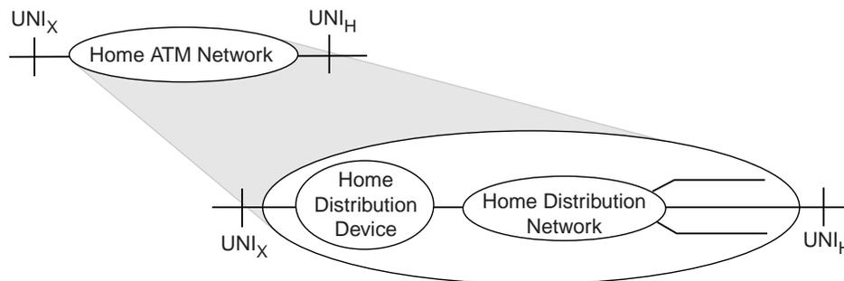
**Figure 1-4 Functional Decomposition of the Home ATM Network**
