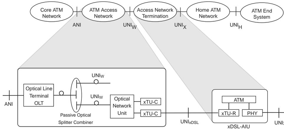
**Figure 3-5 ATM over FTTC/Cab using PON and xDSL Reference Architecture**
