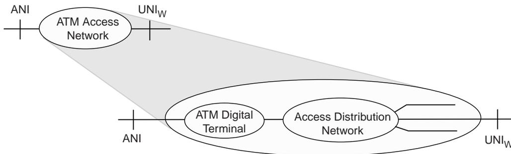
**Figure 1-3 Functional Decomposition of the ATM Access Network**
