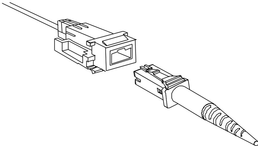
**Figure 3.4.b – MT-RJ Plug and Socket Configuration**
