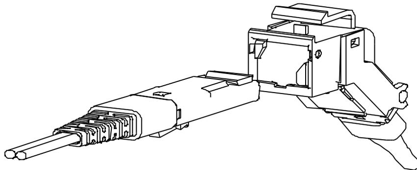
**Figure 3.2.b - SG Plug and Socket Configuration**
