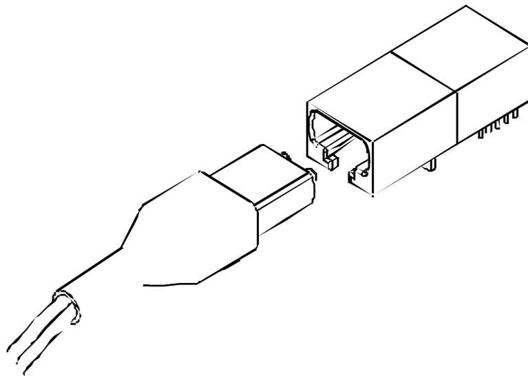
**Figure 3.1.a - Fiber Jack Plug and Receptacle**
