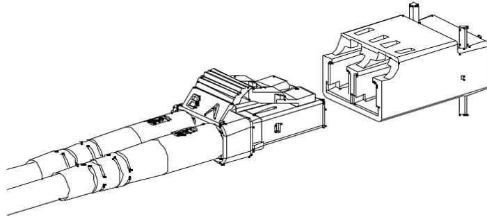
**Figure 3.3.a - LC Interface Configuration**
