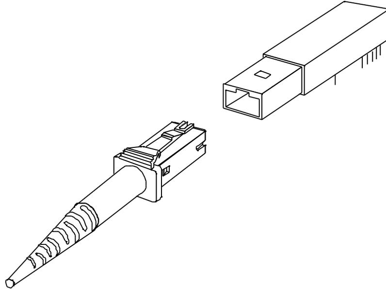
**Figure 3.4.a – MT-RJ Interface Configuration**
