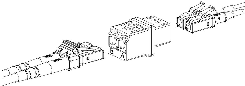
**Figure 3.3.b - LC Plug and Socket Configuration**
